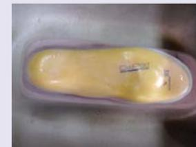
Heat up the cover at 200° degrees for 10 to 15 seconds and shape under the vacuum or directly on the patient's foot.
