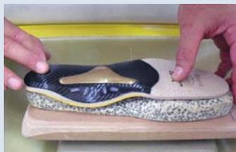
Using a vacuum, place the foot orthotic onto the custom cast.
