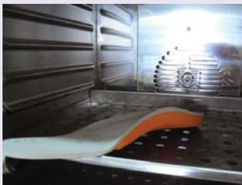
Heat only the parts needing corrections by using an oven at 85-90° degrees for 3 to 4 minutes.
